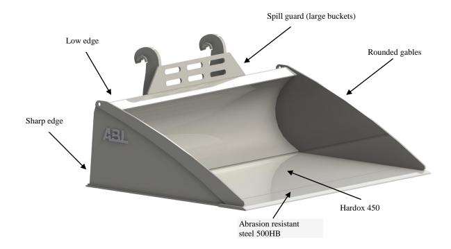
**ABL CE,** can in this range as standard offer different sizes. Widths from **2200mm** to **3100mm** and depths from **1250mm** to **1450mm**. Spill guards on more robust buckets and also a connection for a quick coupler.
